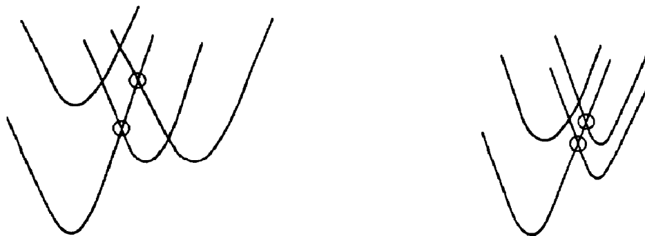
Fig. 2. Effect of the horizontal displacement R and the vertical displacement \Delta E of intermediates on the energy of the crossing point \omega .
